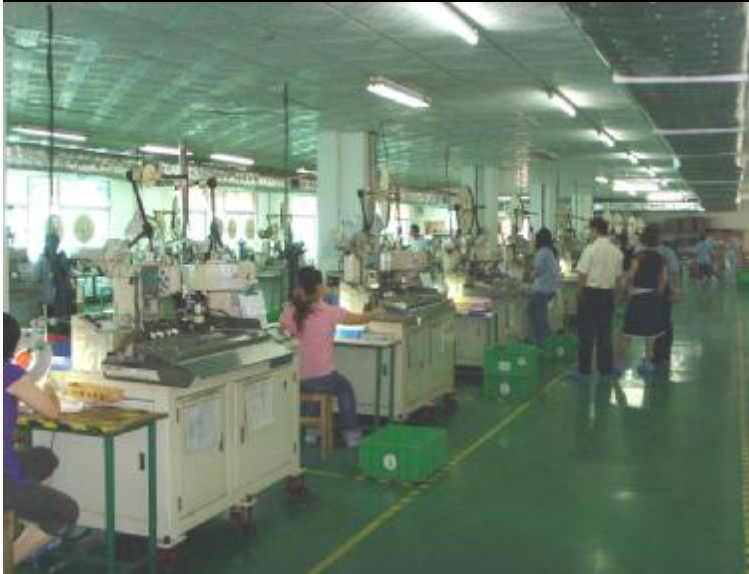
Automatic wire cut, wire stripping, connector assembly and solder dipping production line.
