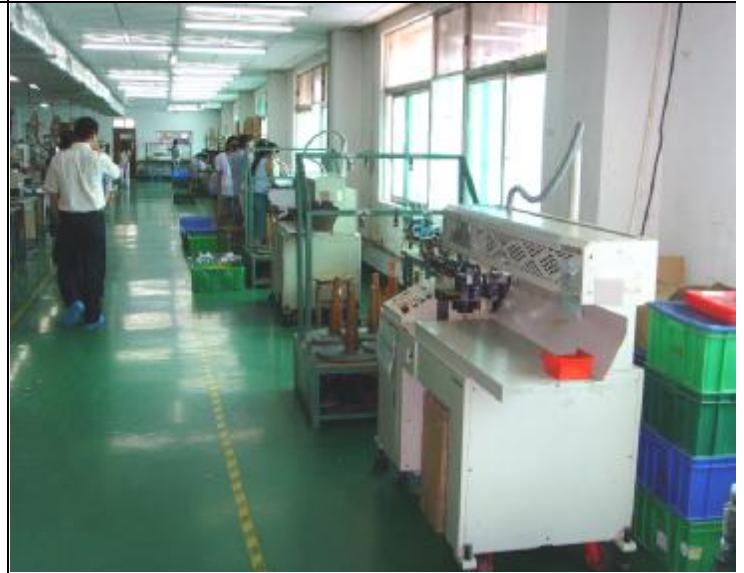
Automatic wire cut and stripping production line- 6 wires cut in one time.
