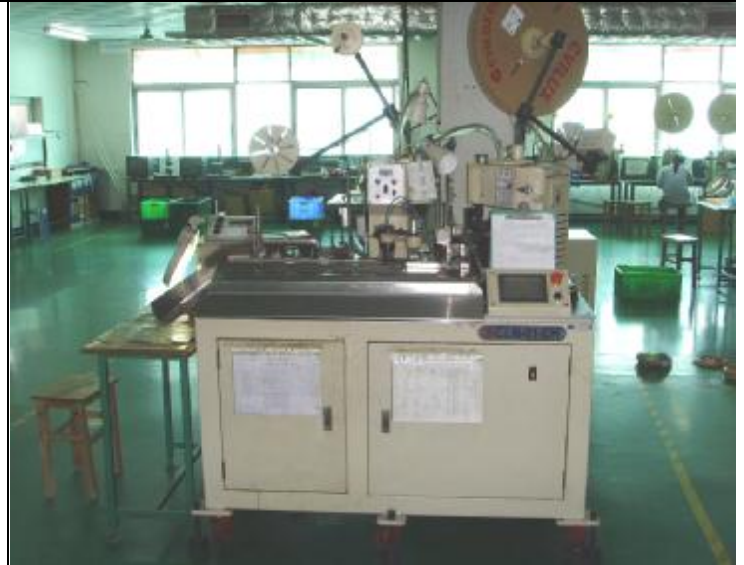
Automatic wire cut, wire stripping, connector assembly and solder machine.
