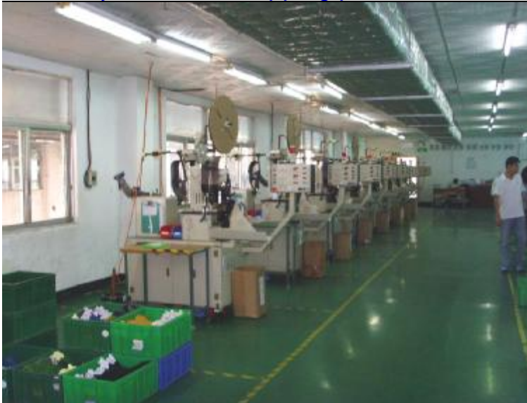
Automatic wire cut, wire stripping, connector assembly production line.
